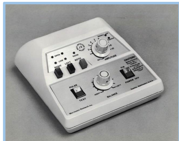
Figure 3. The second production model J3 from 1977. The overclosure switch was deemed unnecessary, but the same three-lead configuration was retained.
