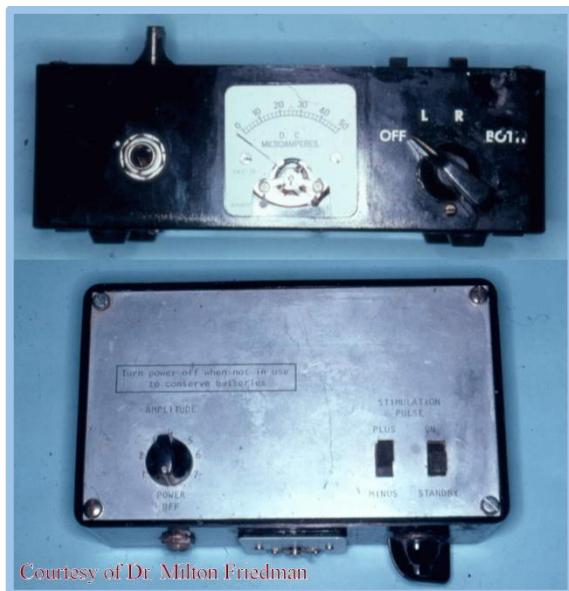
Figure 1. The first prototype of the Myo-Monitor was a very simple device emitting simultaneous left and right 2-millisecond pulses every 1.5 seconds.
